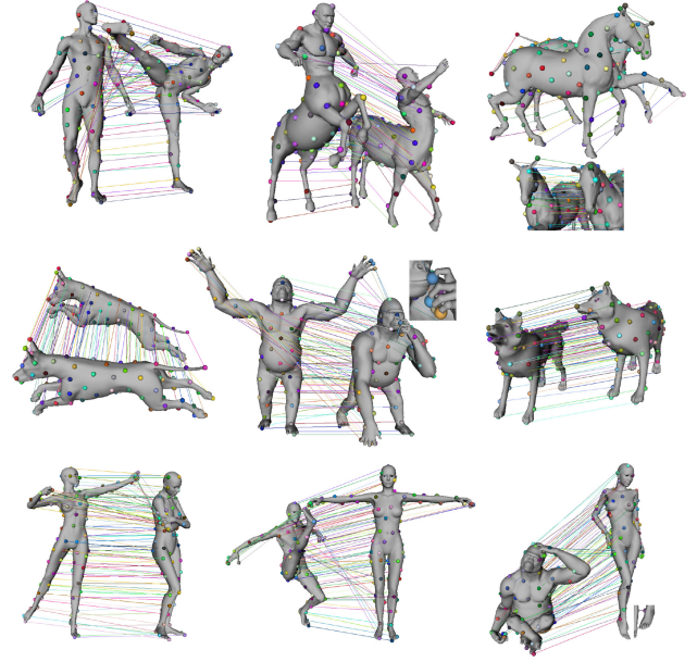
Fig. 10. Resulting genetic maps on the TOSCA set. David to Victoria map shows success for a nearly isometric pair. When isometry deviates significantly, we observe failure, e.g., from the short legs of Gorilla to Victoria .
