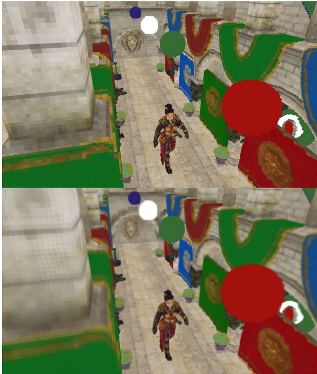
Fig. 8 Comparison of nearest filtering (top) and 8-neighbor filtering (bottom). Images are generated using ray-tracing over the respective sparse voxel octrees
