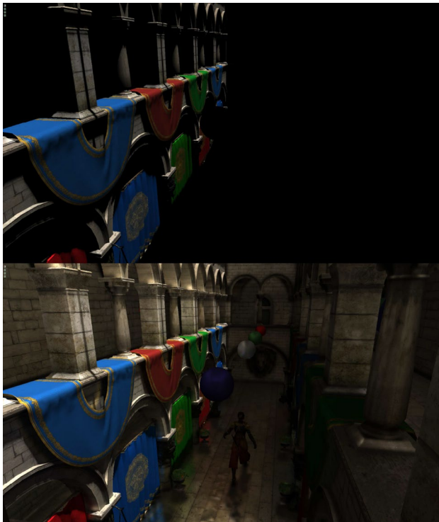
Fig. 6 Comparison between direct illumination (top) and indirect illumination sampled using transformed voxels (bottom). Scene is the modified Crytek Sponza Atrium scene with a single skeletally animated mesh. Sampling is done using the sparse voxel octree
