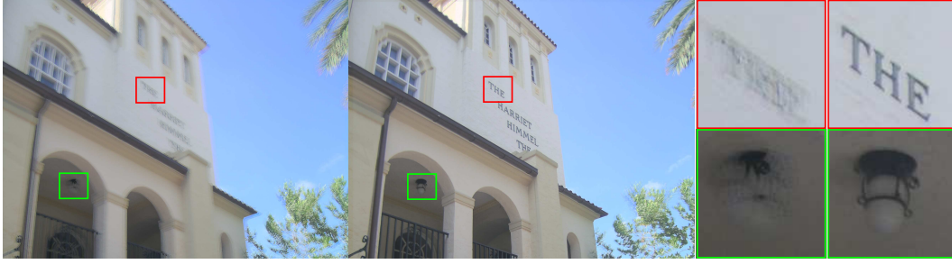
Figure 2: The constituent exposures of the middle image are aligned by using our algorithm with a correlation map size of 32 pixels and a search diameter of 80 pixels in each dimension. The hand-held bracketed sequence contained 5 exposures.
