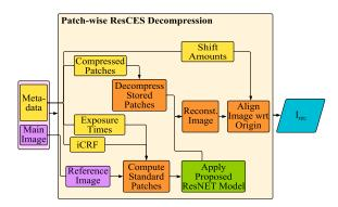
FIGURE 9. The decompression pipeline of the ResCES algorithm.
