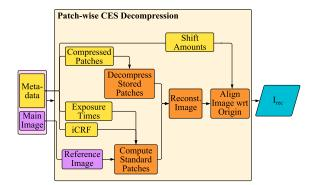
FIGURE 5. The decompression pipeline of the patch-based CES algorithm.
