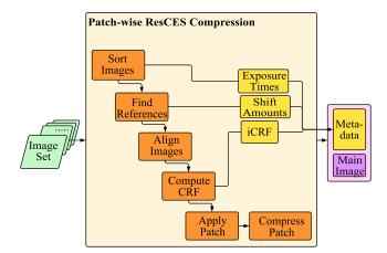
FIGURE 2. The compression pipeline of the patch-based CES algorithm.
