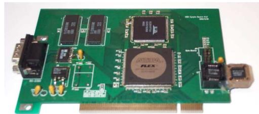
**Fig. 18. Photograph of the RTDS board.**
