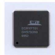
**Fig. 16. Photograph of the crypto processor.**
