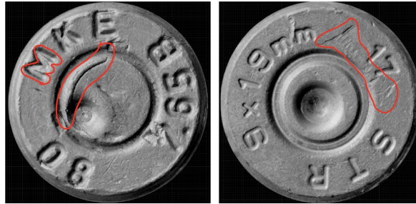
Figure 2: Left: Marks on the cartridge case caused by factory production, such as the headstamp marks of the Mechanical and Chemical Industry Corporation (MKE) of Türkiye. Right: Marks on cartridge cases fired from firearms of the same brand group can be misinterpreted as originating from the same firearm.
