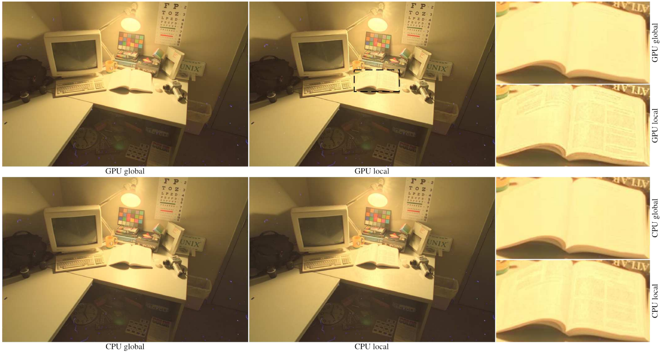
Fig. 7: Global (left) vs. local (middle) tone mapping. As can be seen in the close-ups, the local operator better preserves the visibility of details. The top row shows the results obtained by our GPU implementation, whereas the bottom row shows the results of a reference CPU implementation (Mantiuk et al 2007).
