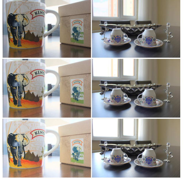
Fig. 5: The left column depicts the tone mapping results with increasing key value in each row (0.18, 0.36, and 0.72 from top to bottom). The right column, on the other hand, depicts tone mapping results with decreasing burn-out threshold ( 10^6 , 5, and 2 from top to bottom).
