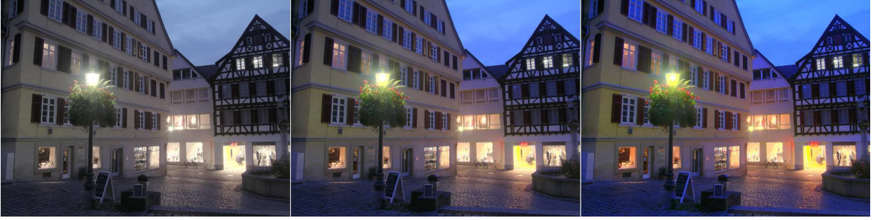
Fig. 6: The effect of changing the saturation parameter. The image on the left has the saturation parameter set to 0.5 and the image on the right to 1.5. The center image has no post tone mapping saturation adjustment (i.e. parameter set to 1.0).
