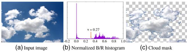
**Figure 7:** This input image (a) has a bimodal normalized B/R histogram (b). As the standard deviation of the normalized ratio image was greater  $T_s = 0.03$ , MCE thresholding was applied to obtain the cloud mask in (c).
