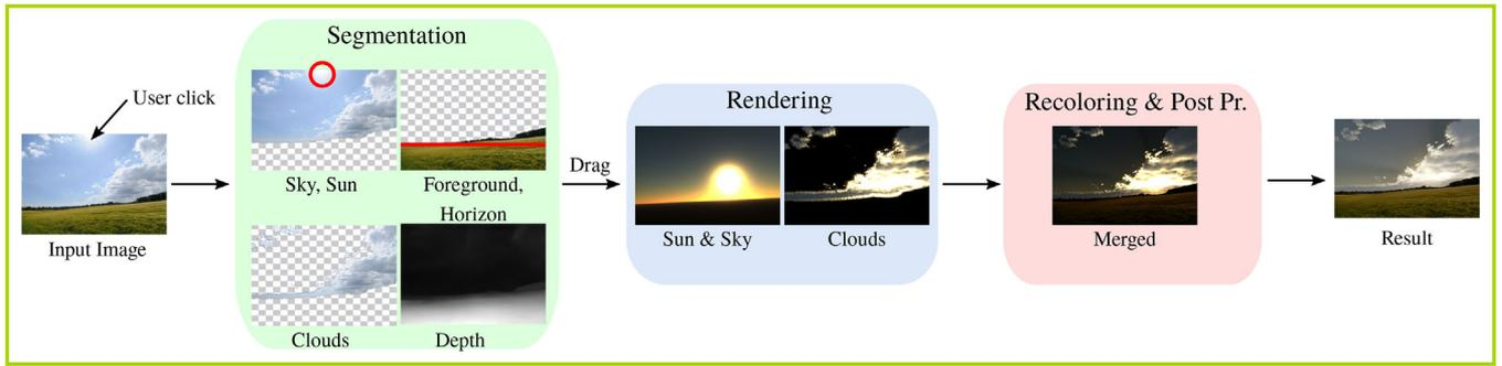
**Figure 2:** The main workflow of our algorithm: the input to our algorithm is a single image. With the user clicking on the sun position, we perform a series of computations to segment important information about the image. Then as the user drags the sun across the sky, atmospheric scattering and cloud rendering are simulated. Finally the results are merged, post-processed, and tone mapped for display purposes.
