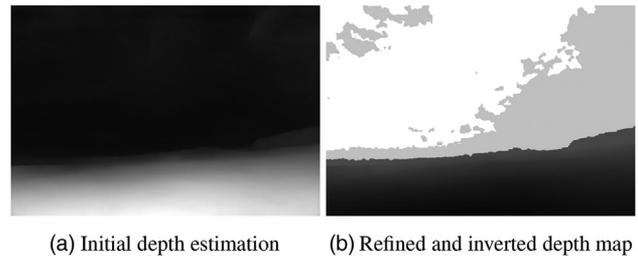
**Figure 10:** We recompute the input depth map (left) so that the most distant object is the sun, followed by the sky, clouds, and the foreground. Note that depth values are inverted in the final depth map (right) so that more distant pixels have higher values.
