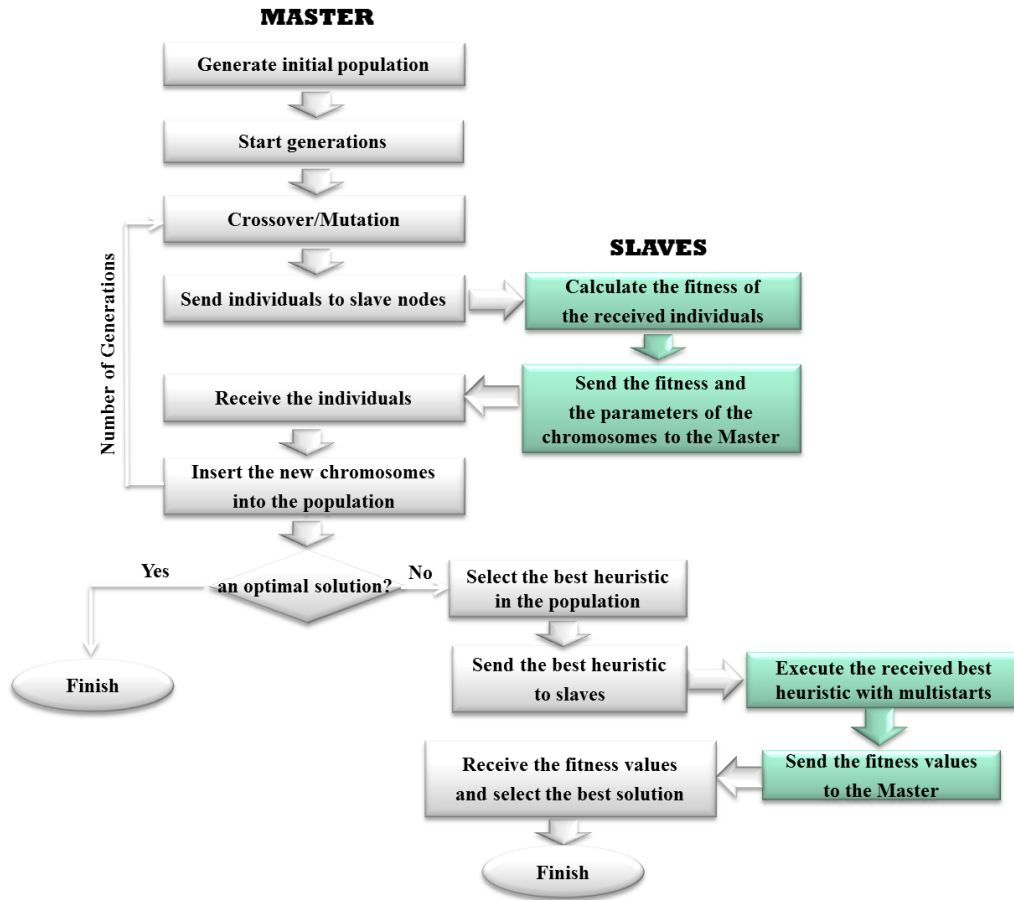
Figure 1: Flowchart of the MSH-QAP algorithm (green boxes are executed at the slaves).
