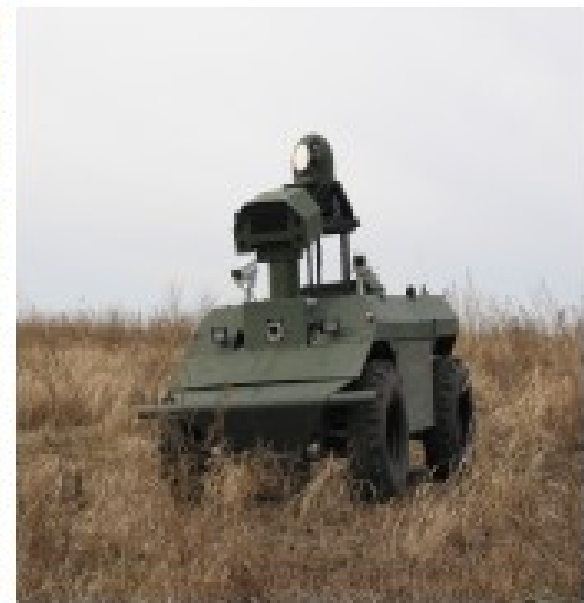
Figure 1. ( left, center ) Multi-resolution Field D* produces direct, low-cost paths (in blue/dark gray) through both high-resolution and low-resolution areas. ( right ) The GDRS XUV robot used for autonomous navigation of outdoor terrain. Multi-resolution Field D* was initially developed in order to extend the effective range of rugged outdoor vehicles such as this by one to two orders of magnitude.
