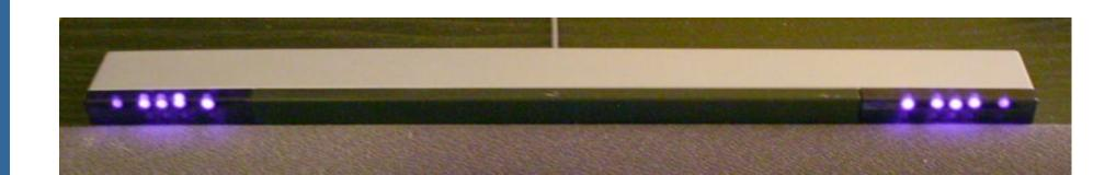
Wii sensor bar has strong infra red LED's, which creates a big glaring point for the IR camera to detect.
