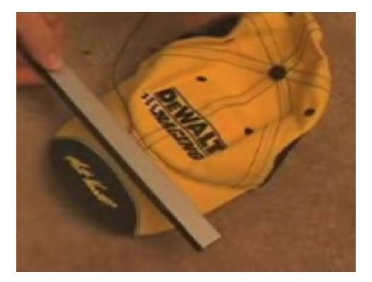
Putting the sensor bar on a cap is a simple solution for head tracking.
