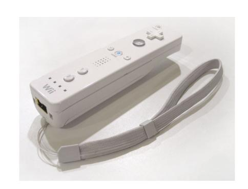
Wii remote will be used as an infra red camera. Also other infrared camera's can be used for this purpose. We just use it because we have it already, and wii remote does the point position extraction for us. The downside is it can only extract 4 point positions.
