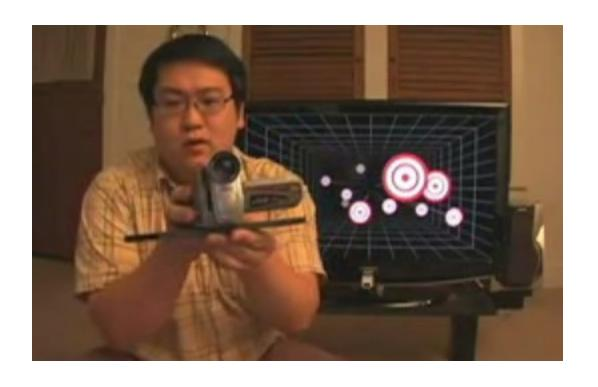
Johnny Lee holding the sensor bar, below the camera, so that wii remote tracks the position of the camera, and the image on the TV is generated accordingly.
