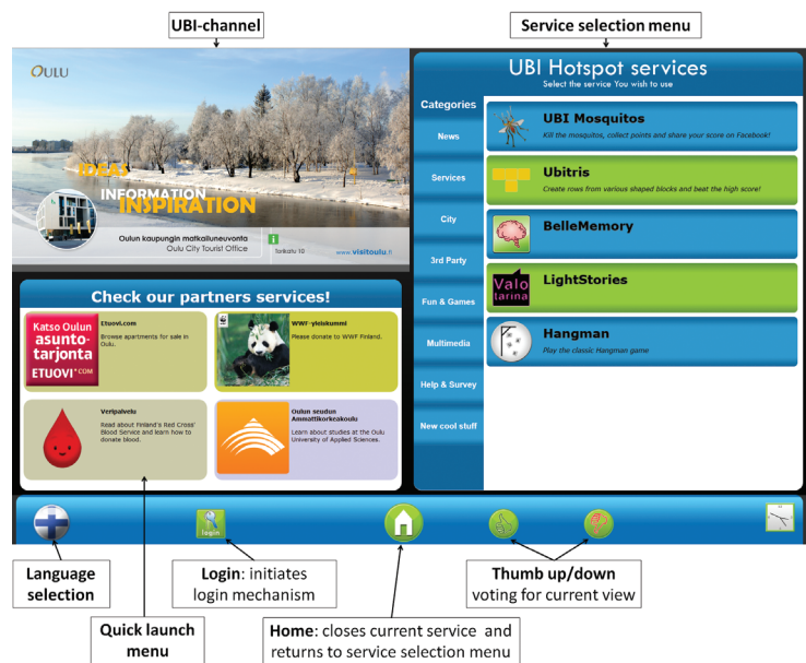
Figure 2. Version 3 of a hotspot in interactive mode. The screen is split between the UBI channel (top left), a customizable multimedia playlist; the quick-launch menu providing one-touch access to selected services (bottom left); and the UBI portal (right) through which users can access 25 services in seven categories, as well as a help and survey category.
