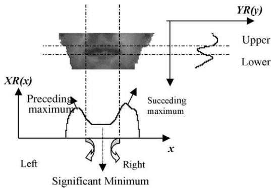
Fig. 3. Y- and X-Relief characteristics of mouth.
