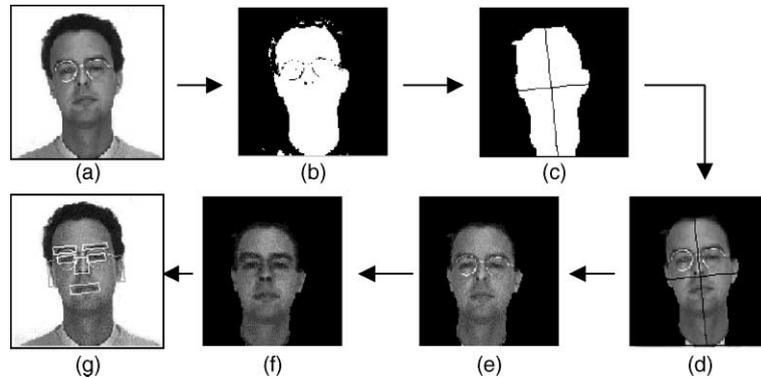
Fig. 1. (a) Original input image, after (b) Skin Filter-1, (c) connected components labeling, closing and ellipse fitting, (d) grayscale image multiplied by the silhouette image, (e) head normalization, (f) grayscale erosion, and (g) the output of facial feature segmentation.
